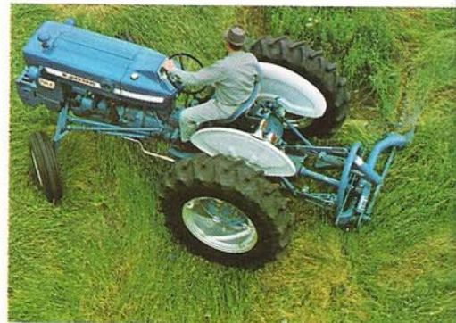
Short 77.3-in. wheelbase makes tight turns easy.
