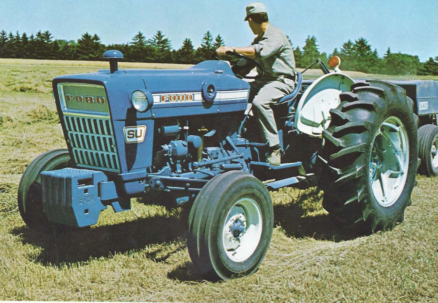
Independent PTO comes standard on the Ford 4000 SU.
