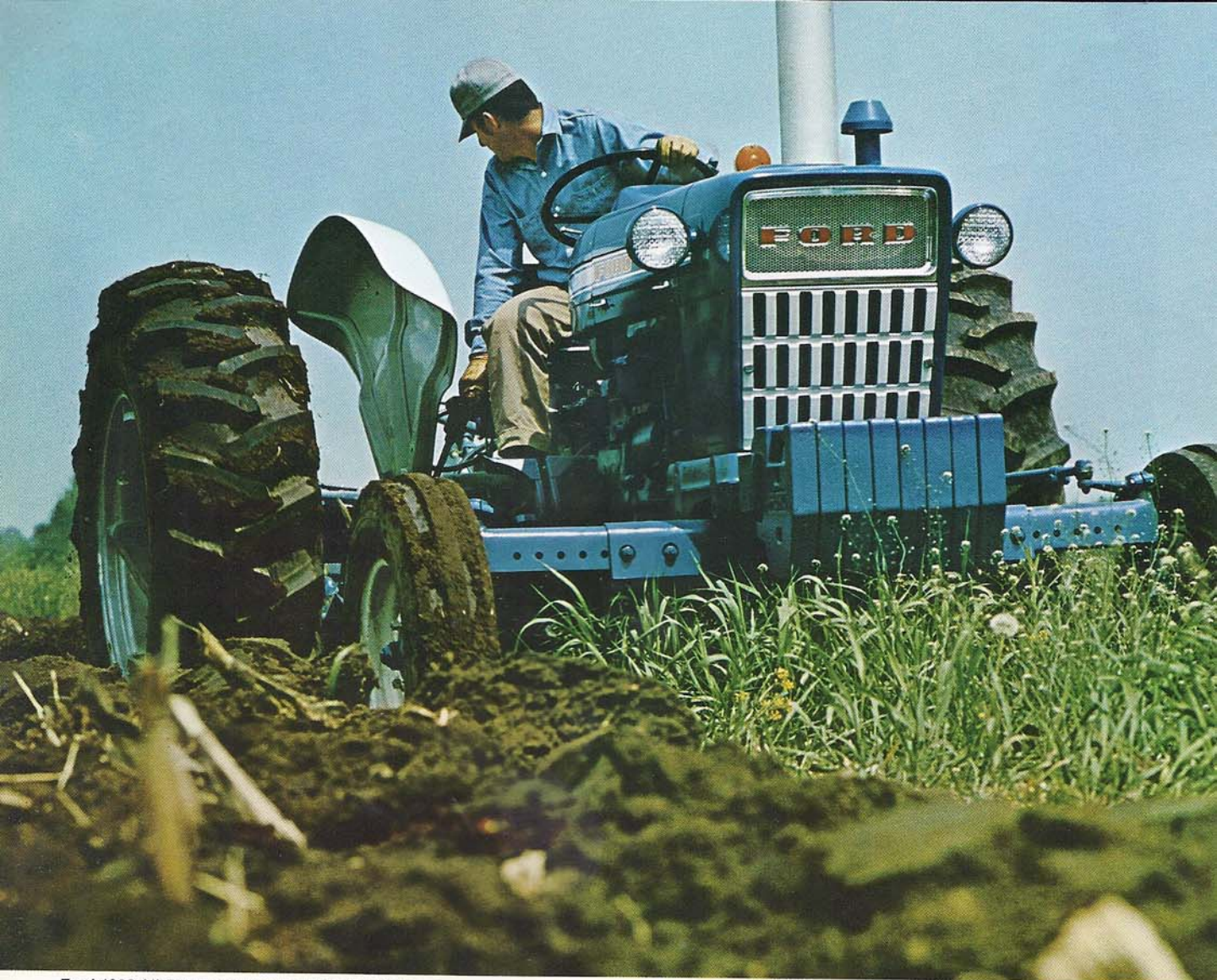
Ford 4000 All-Purpose can plow up to four furrows.
